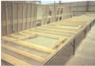
Panelized walls, floors, and roofs are factory-built and assembled on site (courtesy, SWA).
